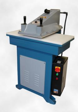
The machine is used for cutting out parts of various shapes from leathers, synthetic materials, rubber, paper etc. by cutting die.
