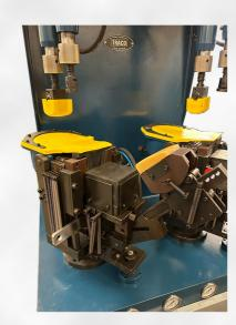
The machine is designed for pressing (adhesive bonding) soles to a shoe upper, which was lasted over the last. The soles can be adhesive bonded to the men's, ladies' and children's footwear, and also to the footwear with high heel or to knee high boots.
